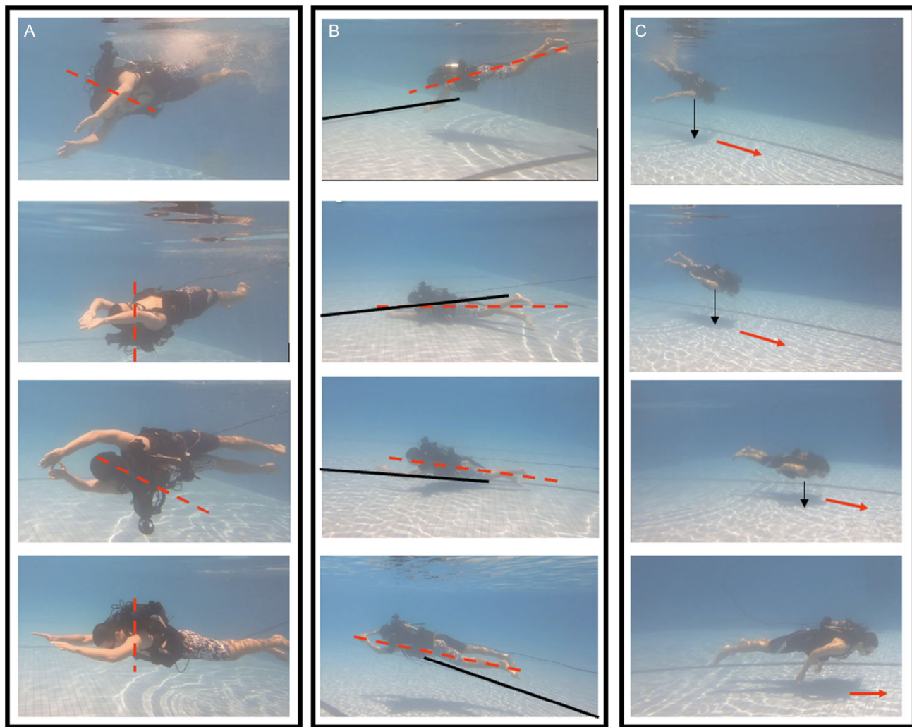
Figure 7. Screenshots of field testing for supernumerary diving assistance without using any of his limbs in a swimming pool. A) Helical cruising to move forward while spinning about his body axis. B) Turning with depth control to turn left while diving to the bottom of the pool. C) Cruising with depth control to move forward while diving to the bottom of the pool.
