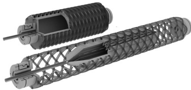
FIG. 1. Concept of FORA. Upper : pressurized state, lower : natural state. The design consists of an inner origamic chamber, an external braided mesh, and connection fittings. FORA, Fiber-reinforced Origamic Robotic Actuator.
