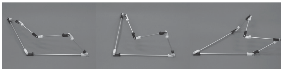
Figure 17. The motion sequence of the type V linkage model.
