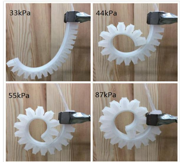
Fig 5. The PAM deformation under different air pressure
