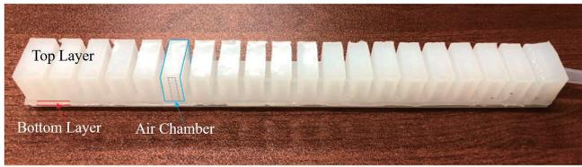
Fig 3. The fabricated PAM
