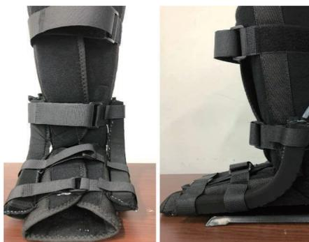
Fig 4. The active orthotic device with two PAM for each foot
