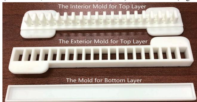
Fig 2. The 3D printed molds
