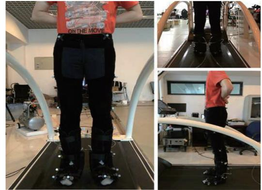
Figure 8. Marker placement and experiment set-up
