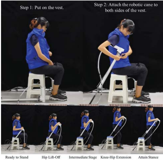
Fig. 4: A two-step setup and demonstration of the robotic cane system in chair. Here, the operator use hand to actuate the robotic cane by pushing a button on the handle instead of using hands for upper body support.
