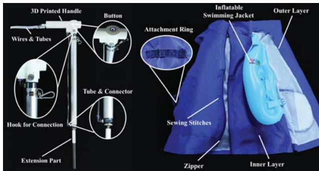
Fig. 5: The proof-of-concept prototype: a redesigned air cylinder as the robotic cane and a swimming jacket enclosed in the vest.
