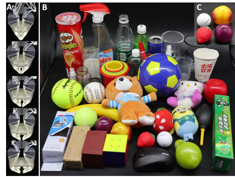
Fig. 5: Fast calibration for gripper in a real application (A). A selection of sorting objects are selected from the YCB dataset and daily objects (B). Due to the parallel finger configuration used in our experiment, some objects (C) may slip through the gap between dual-fingers during grasping.
