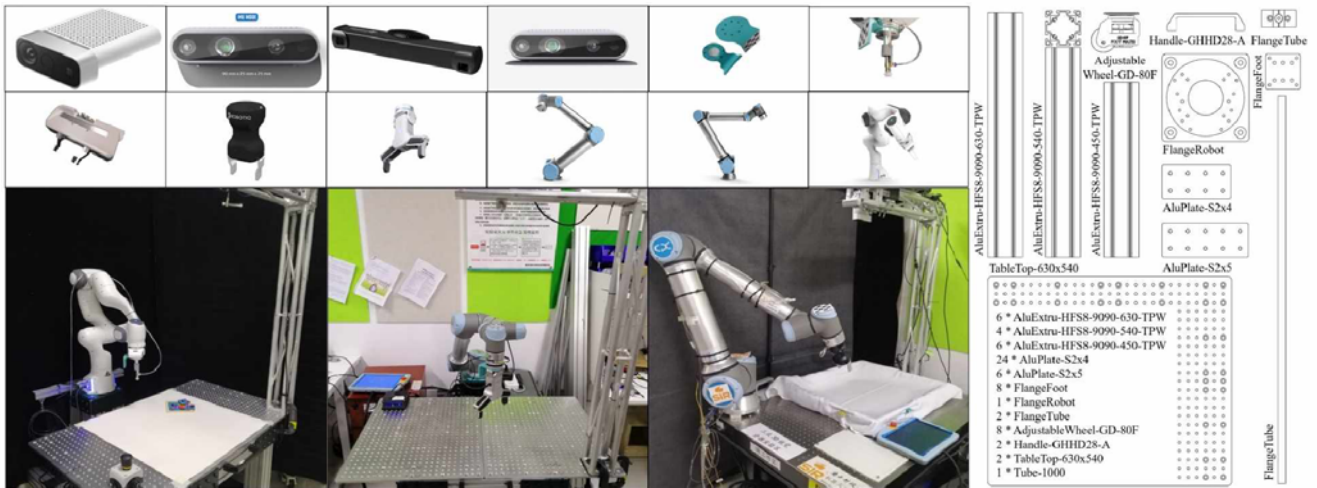
Fig. 2: Design overview of the robotic hardware in DeepClaw, including the supported cameras, end-effectors, and robotic manipulators (top), the three robot cells used in this papers (bottom), and the all the mechanical parts for a full assembly (right).
